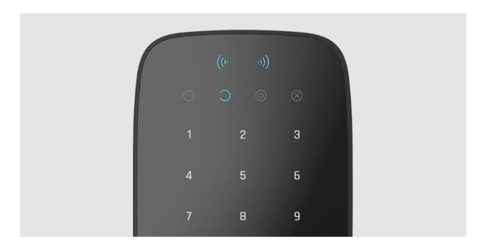
You can use the KeyPad Plus without ambient lighting as the keypad has a backlight. The pressing of the buttons is accompanied by a sound signal. The backlight brightness and keypad volume are adjustable in the settings. If you do not touch the keypad for 4 seconds, KeyPad Plus reduces the backlight brightness, and 8 seconds later goes into power-saving mode and turns off the display.
